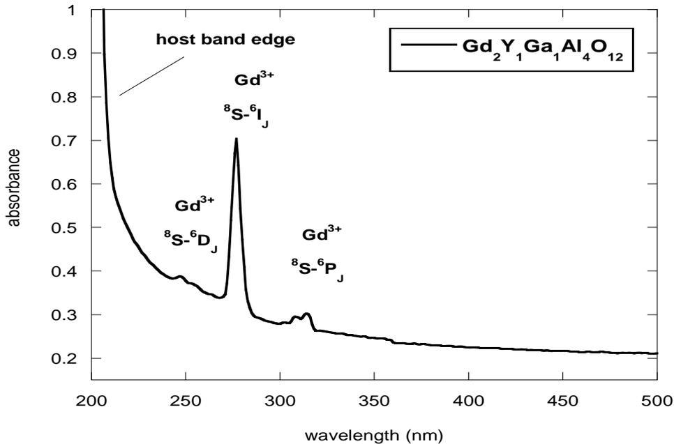
Absorption spectrum of  $Gd_2Y_1Ga_1Al_4O_{12}$ . Intense  $Gd^{3+}$ -related peak at 270 nm as well as host lattice absorption region ( $\lambda \leq 220$  nm) are evident.
