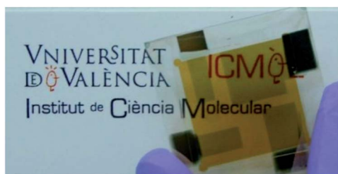
Fig. 5 Photograph of the semitransparent solar cell having a 100 nm perovskite layer resulting in an AVT \sim 30% and a PCE of 6.4%.
